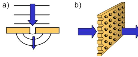
a) Single hole transmission is very small b) Transmission through a number of holes and intensity is higher when normalized to total area
